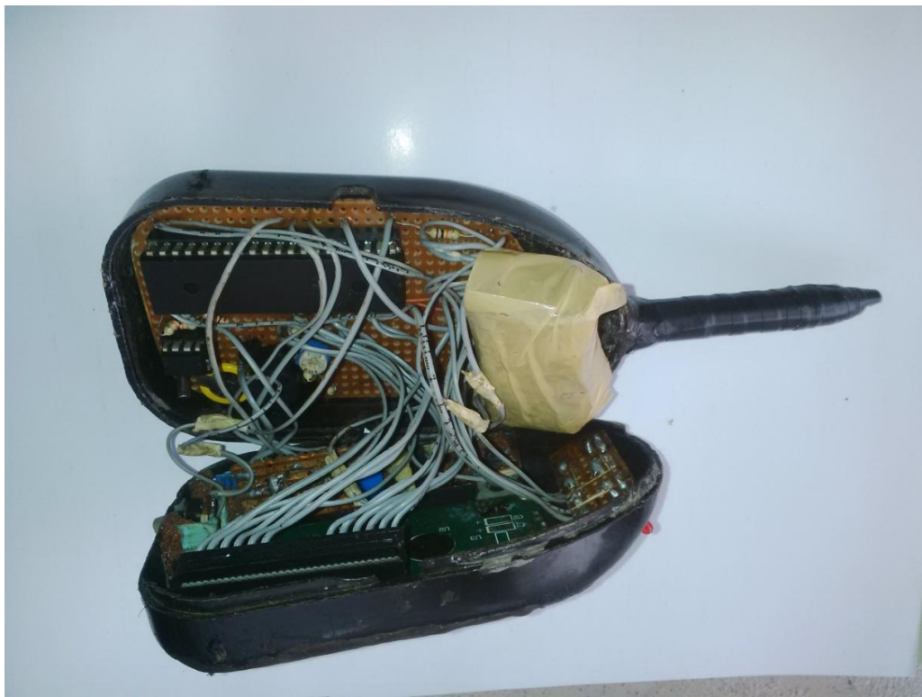
Figure 4: Implementation of the electronic thermometer
