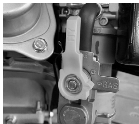
Switch to Gas position
